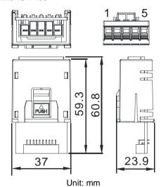
Pin no. AS-F2AD AS-F2DA AS-F422 AS-F485 1 V1+ VO1 R+ 2 11+ IO1 R-3 V2+ VO<sub>2</sub> T+ D+ 12+ 102 T-4 D-COM COM SG SG
