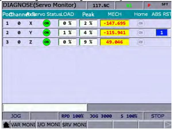
3: A system can run absolute reset only in **JOG** or **MPG** mode. Move the mechanical position of the axis with JOG or MPG operation to the proper location, press key [1] then press the **Enter** key to finish the absolute reset. The origin status indicator lights up, the mechanical coordinates reset to 0, and the axis returns to the origin.
