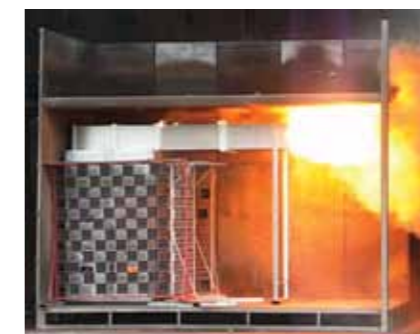
Internal arc fault test, 31.5kA/1s
